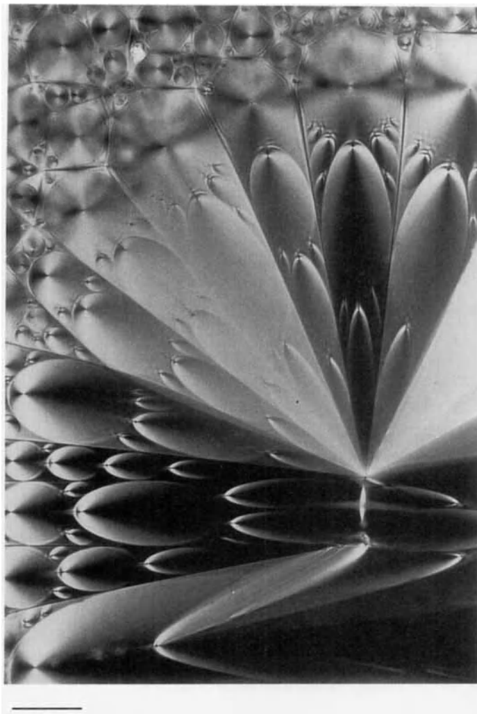
Figure 33. Polygonal field (top left) and elongated polygons, with their long edges converging at a +\pi disclination. 4-Cyano-4'- n -octylbiphenyl plus Canada balsam; crossed polarizer. Scale bar: 50 \mu\text{m} .
