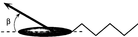
Figure 4. Schematic of a mesogen with an off-axis dipole moment making an angle of \beta with the molecular long axis.
